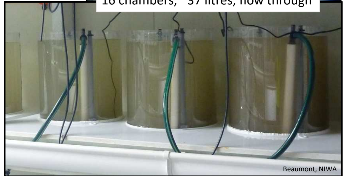
Suspend sediments, control loading 16 chambers, ~37 litres, flow through
