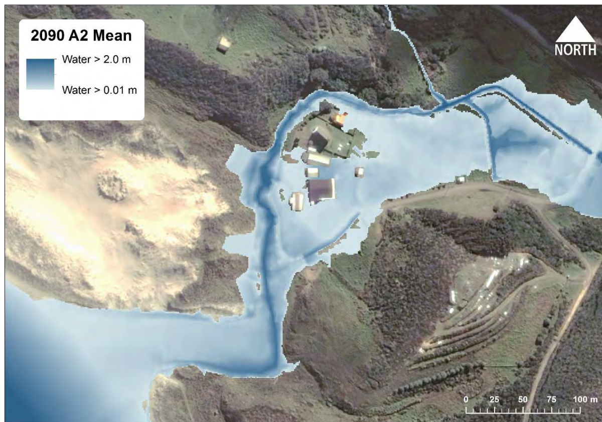
Figure 16: Modelling climate change induced coastal- stream reach flooding for 2040 and 2090 AD around the Mātihetihe Marae complex under the A2 'mean' climate change scenario and sea-level rise scenarios as described in the text.
