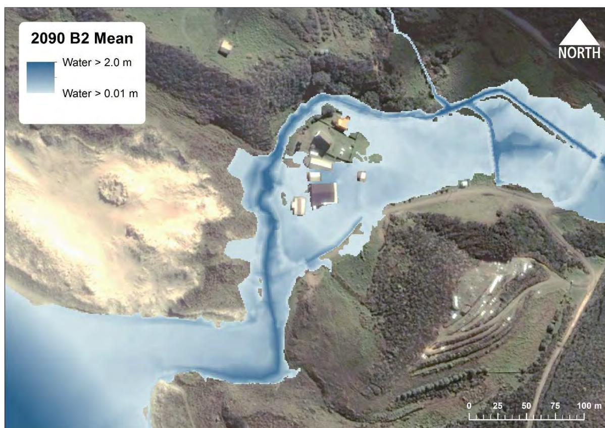
Figure 15: Modelling climate change induced coastal-stream reach flooding for 2040 and 2090 AD around the Mātihetihe Marae complex under the B2 'mean' climate change scenario and sea-level rise scenarios as described in the text.
