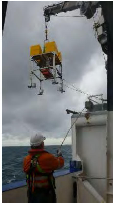
Figure 4-24: Image from the cut-away on RV Tangaroa while deploying a benthic lander.
