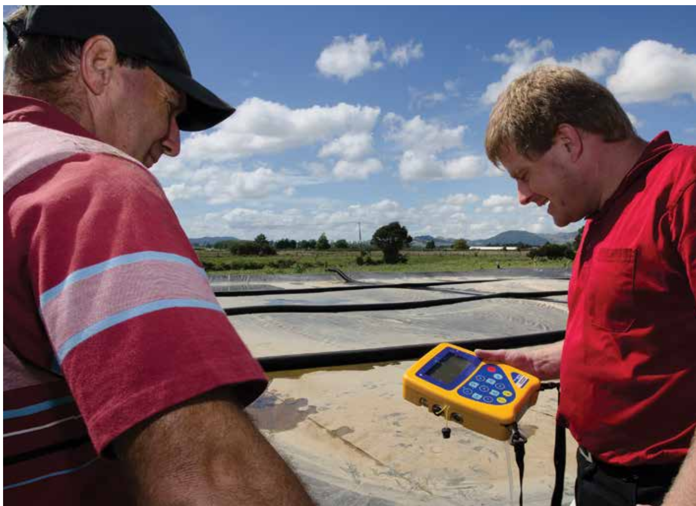
Farmer Neville Barr (L) and NIWA resource engineer Stephan Heubeck use a gas analyser to measure levels of methane, carbon dioxide, hydrogen sulphide and oxygen from the covered anaerobic digester pond. (Dave Allen)
