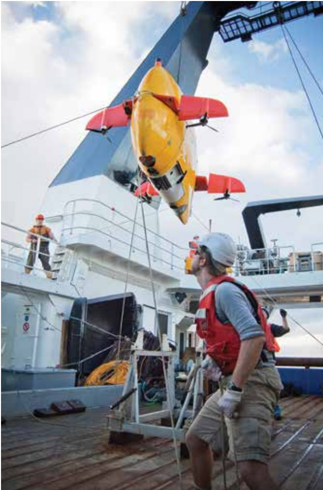
Capable of reaching a depth of 6000 metres, Woods Hole's 'Sentry' is readied for deployment from Tangaroa . The AUV (Autonomous Underwater Vehicle) uses multibeam and sidescan sonars to map the topography and capture thousands of photographs of the seafloor. (Rob Stewart)
