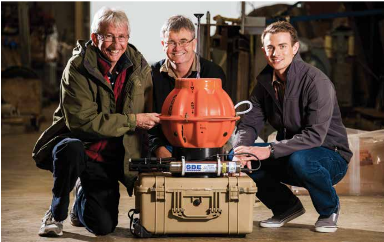
NIWA Physical Oceanographer Philip Sutton (centre), Dean Roemmich, Professor of Oceanography (left), and Kyle Grindley, Development Engineer, from Scripps Institution of Oceanography in San Diego, California, with a deep Argo float ready for deployment near the Kermadec Trench. (Dave Allen)
