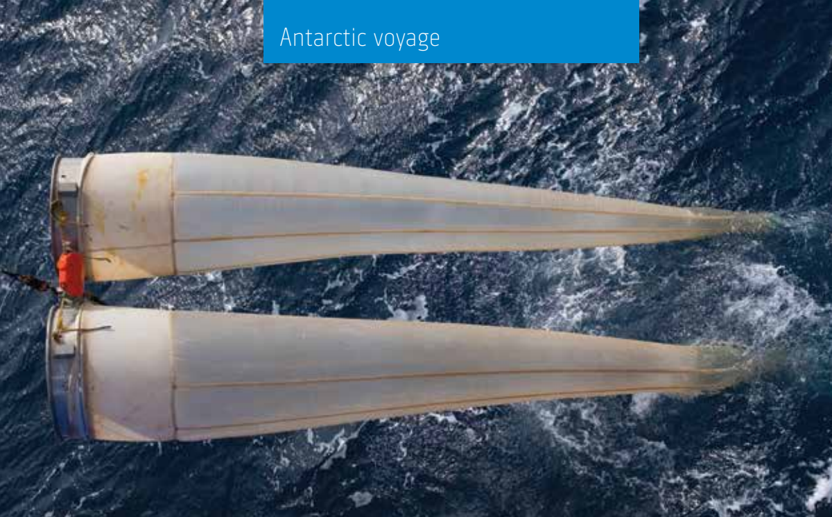
Top: 'Bongo' nets can be deployed as deep as 1000m, enabling researchers to build a detailed picture of the rich range of plankton found in Antarctic waters. (Dave Bowden)
