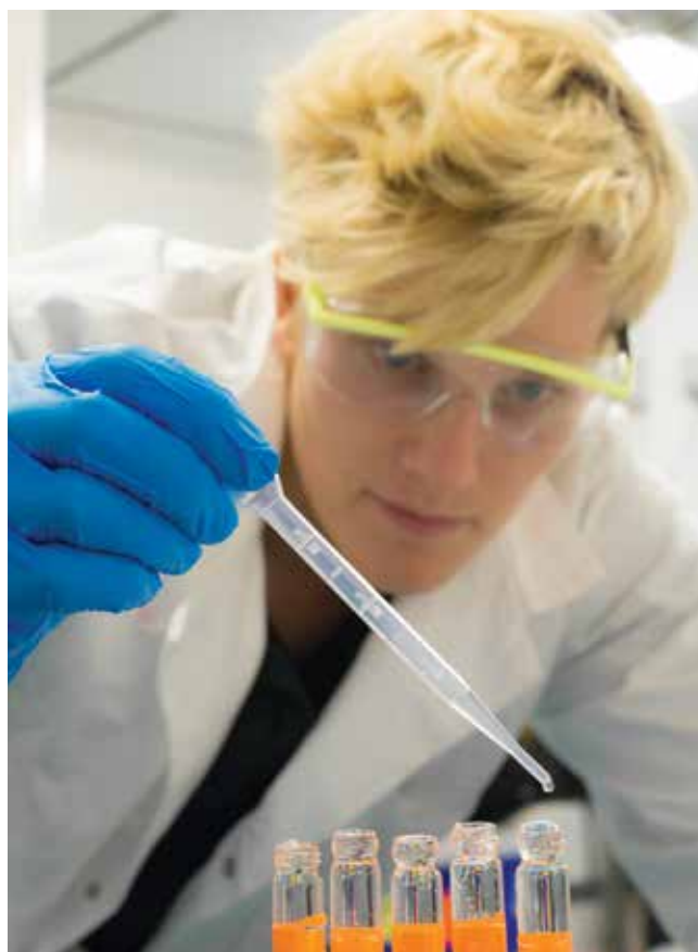
Blake Hornblow adds mercuric chloride to sea water to kill the phytoplankton and stop biological activity in Tangaroa's middle lab. (Dave Allen)
