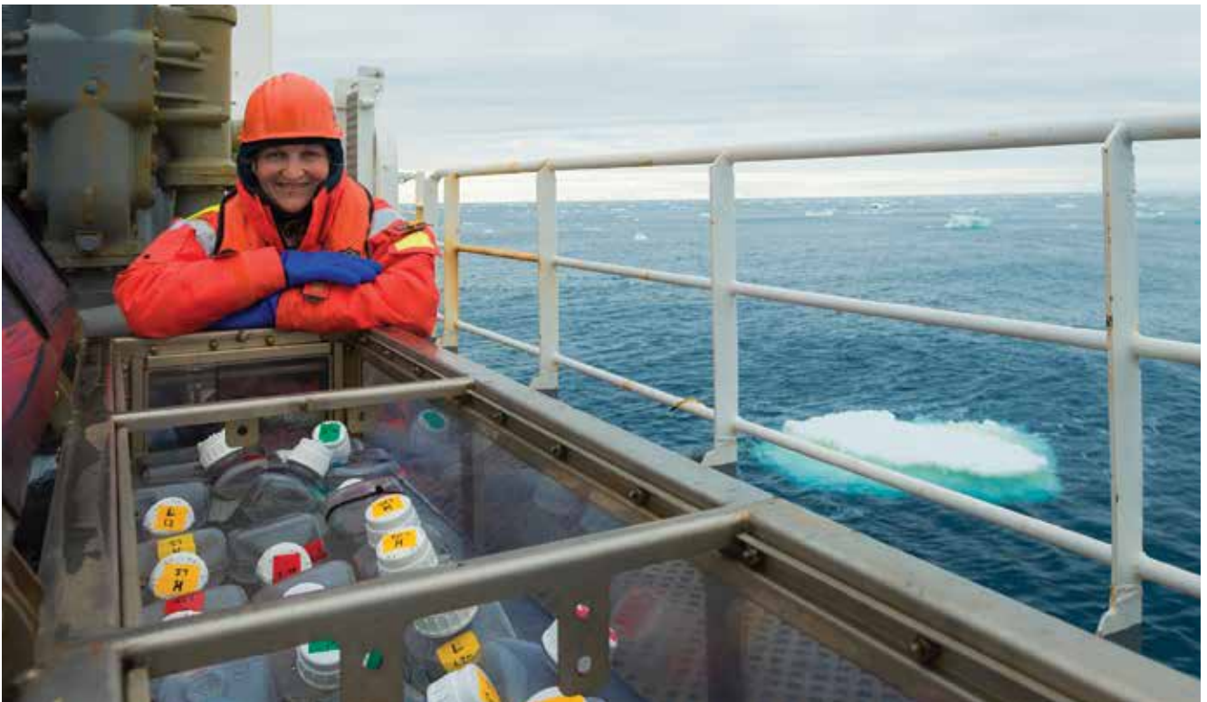
Sarah Bury with one of her seawater incubators – part of an experiment designed to measure phytoplankton nutrient uptake and primary production rates. (Dave Allen)
