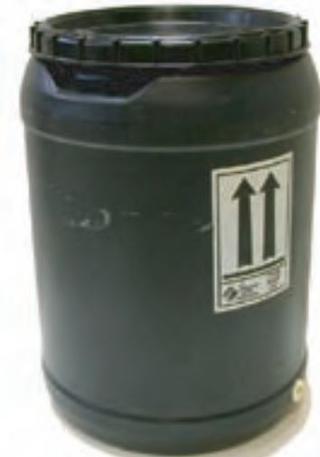
Figure 6.2: Black plastic barrel with secure lid, suitable for storage and transport of formalin-preserved coralline specimens from the field.
