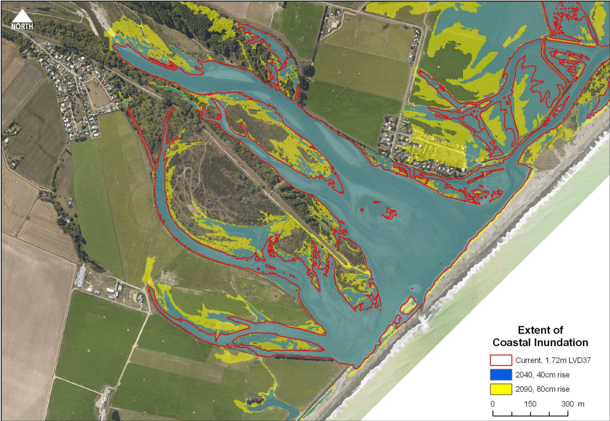
Figure 22: Extent of coastal inundation for current extreme storm-tide conditions (1% AEP) and for climate change-adjusted sea-levels for 2040 AD and 2090 AD.
