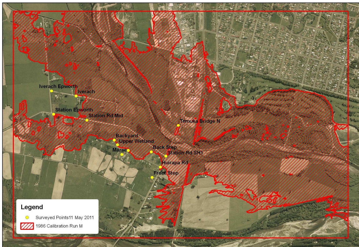
Figure 14: Calibration model results map and surveyed points across the extent of the model domain.
