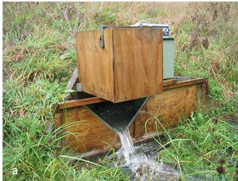
Figure 3.6 SH1 @ Redvale: weir and instrumentation for water level measurement at (a) pond inlet (b) pond outlet
