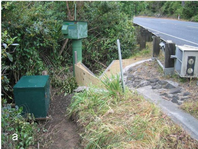
Figure 3.5 SH16 @ Huapai: weir and instrumentation for water level measurement at (a) kerbed site and (b) road drainage channel outlet.
