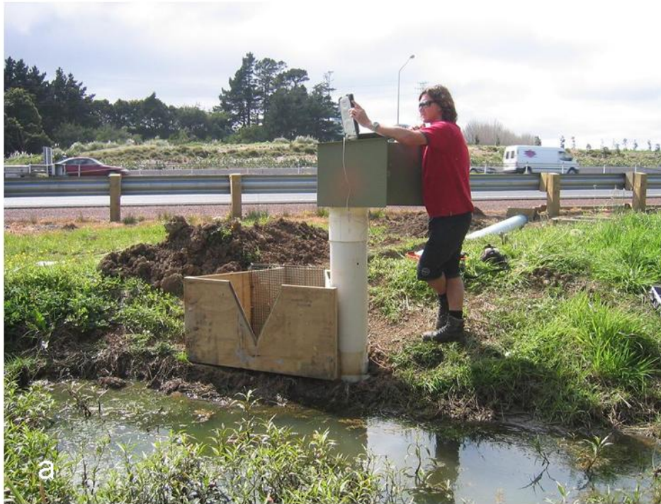
Figure 3.4 SH1 @ Northcote: weir and instrumentation for water-level measurement at (a) kerbed site and (b) inside manhole at swale site
