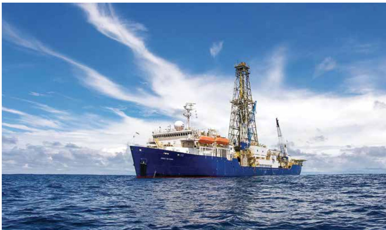
The JOIDES (Joint Oceanographic Institutions for Deep Earth Sampling) Resolution is a specialist research vessel capable of drilling deep into the ocean floor to collect and study core samples. (National Science Foundation)
