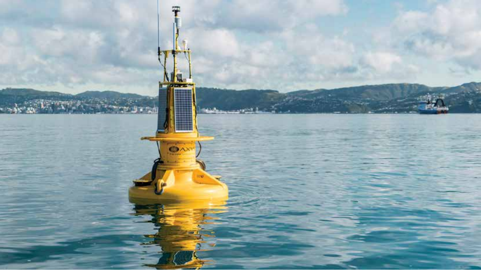
A buoy with the ability to transmit real-time oceanographic and weather data, WRIBO (Wellington Region Integrated Buoy Observations) commences service in Wellington Harbour. (Stuart Mackay)
