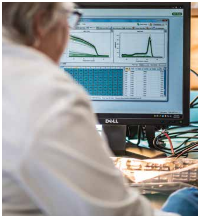
Microbial ecologist Debbie Hulston runs a SYBRgreen assay on the qPCR machine. The test analyses the melting points of amplified DNA to detect the bonamia parasites. The green peaks on the graph indicate positive results for the presence of both Bonamia ostreae and oyster DNA. (Dave Allen)
