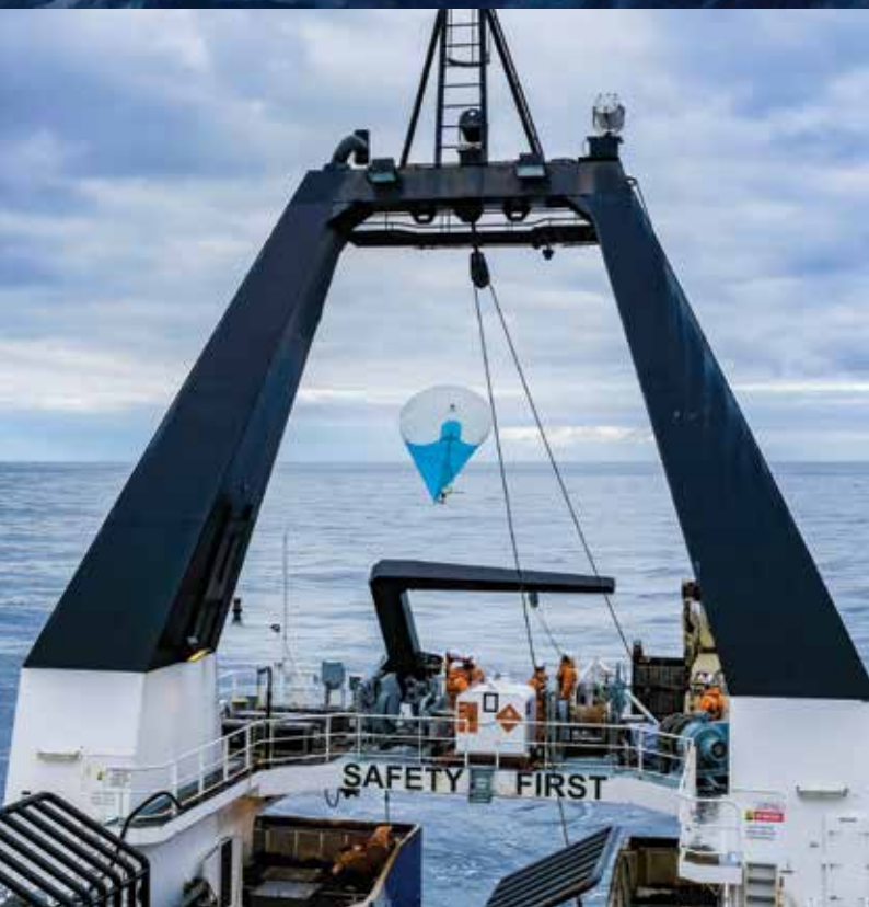
A helikite is deployed from the stern of Tangaroa to measure aerosols, pressure, temperature and relative humidity. (David Bowden)
