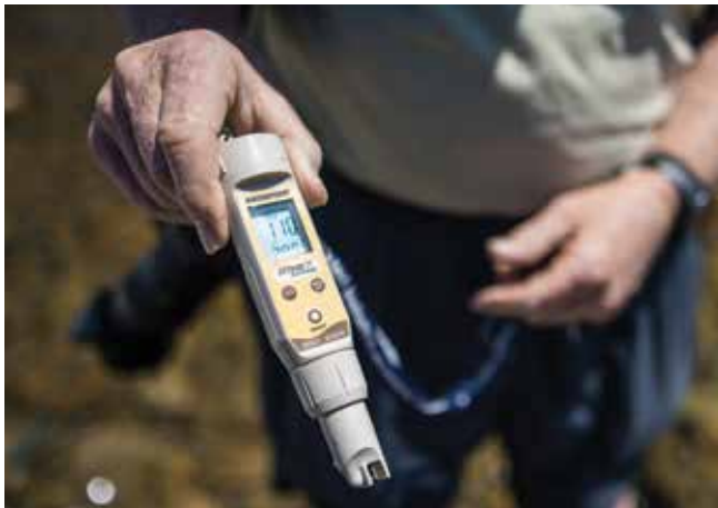
NIWA-provided kits are used to measure various parameters including clarity, conductivity, dissolved oxygen, pH, temperature, nitrates and phosphates. (Dave Allen)
