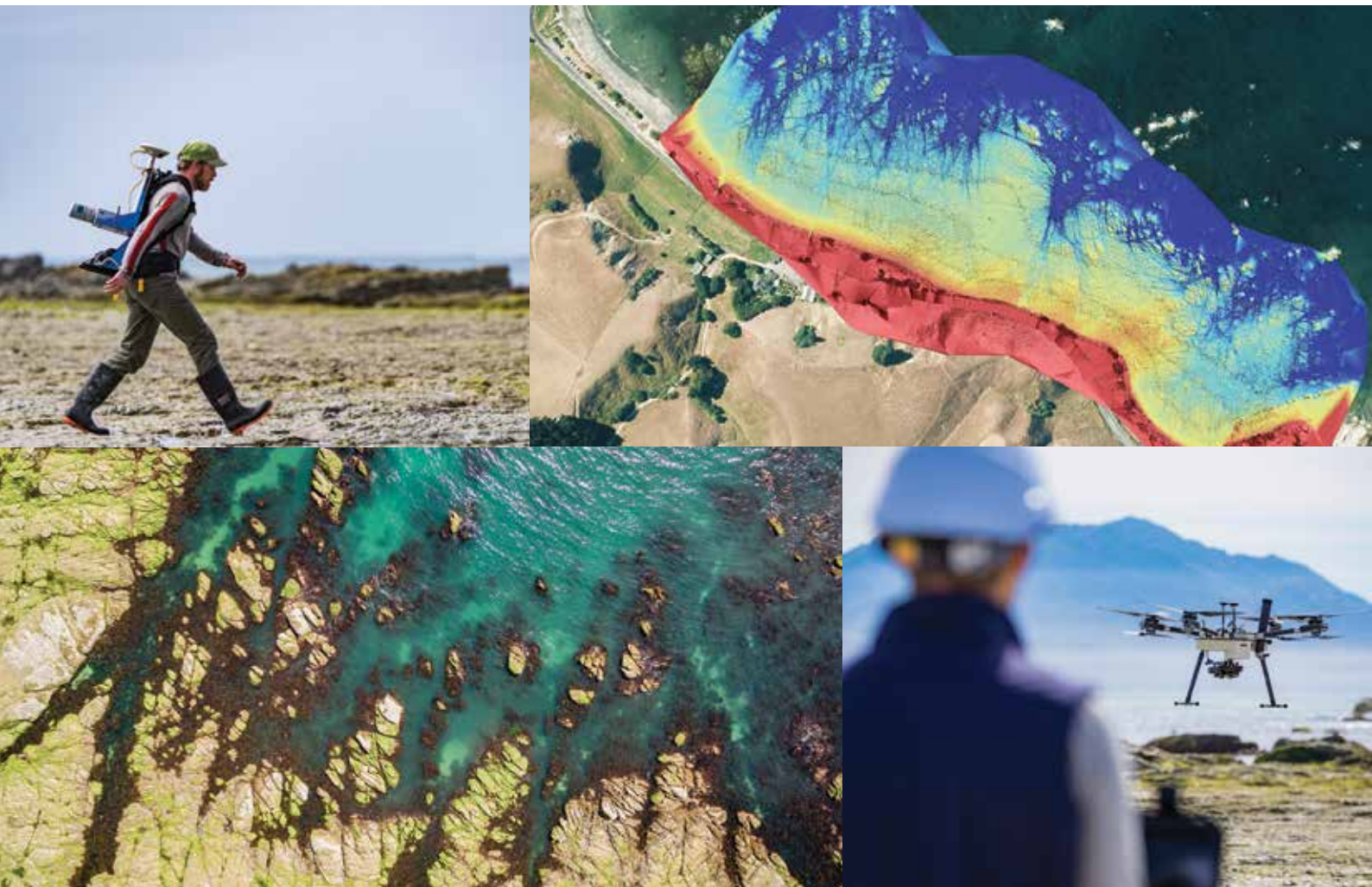
(Top left) GIS Technician Jochen Bind with 'Snoopy' on his back (aka NIWA's Scanlook 2.0 mobile mapping LiDAR system). (Top right) A preliminary rendering, showing a bird's eye view of the data gathered by the LiDAR unit. (NIWA) (Bottom left) A drone's eye view of Kaikoura's uplifted seabed. (Bottom right) David Plew launches NIWA's Altus LRX drone into the survey area, which captures a sequence of high-resolution images that will be used for habitat mapping. (Dave Allen)
