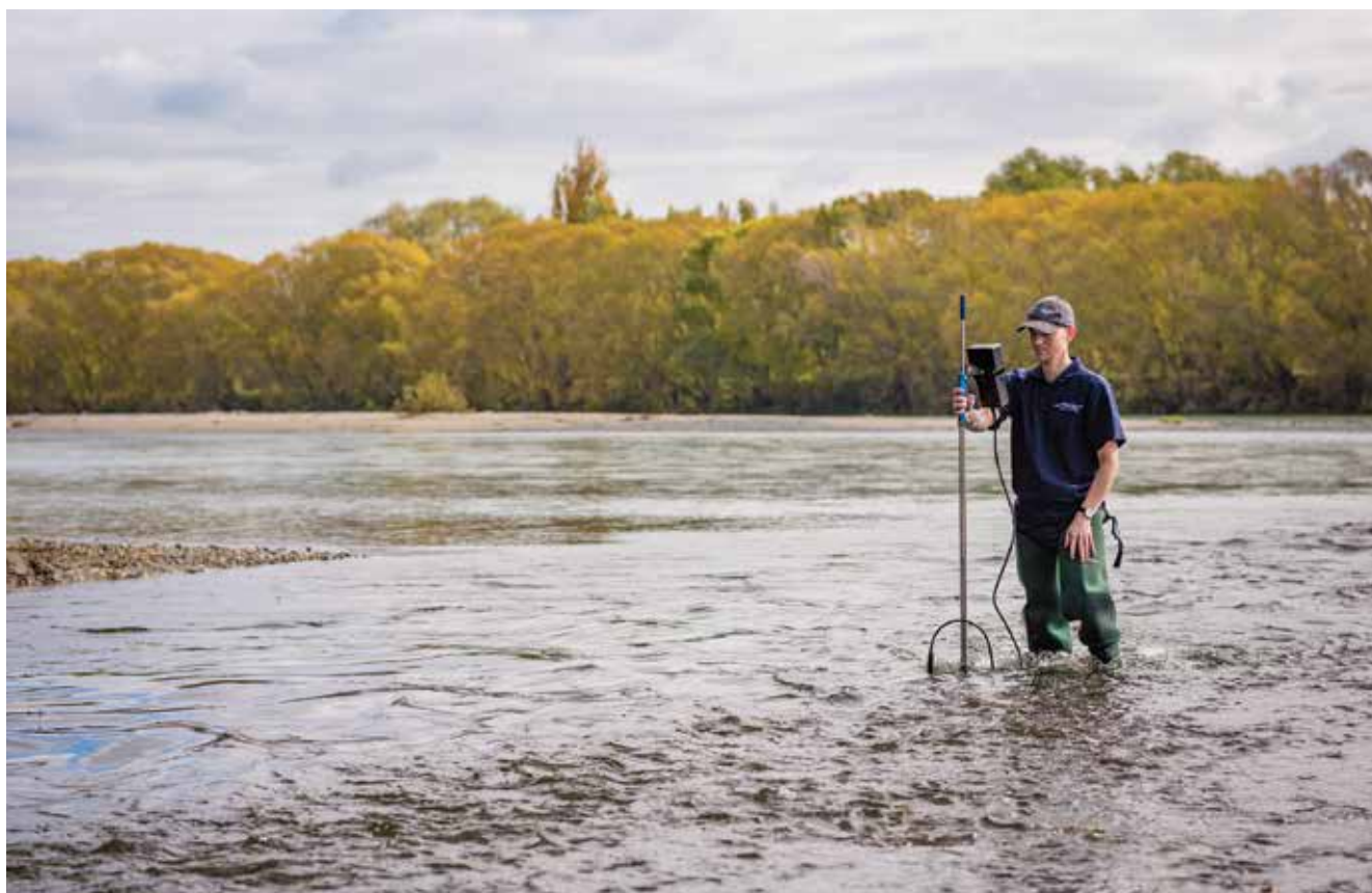
Dr Doug Booker using a Flow Tracker ADV (Acoustic Doppler Velocity) meter. This instrument gives us water velocity at the point where we set it in the water column. (Dave Allen)
