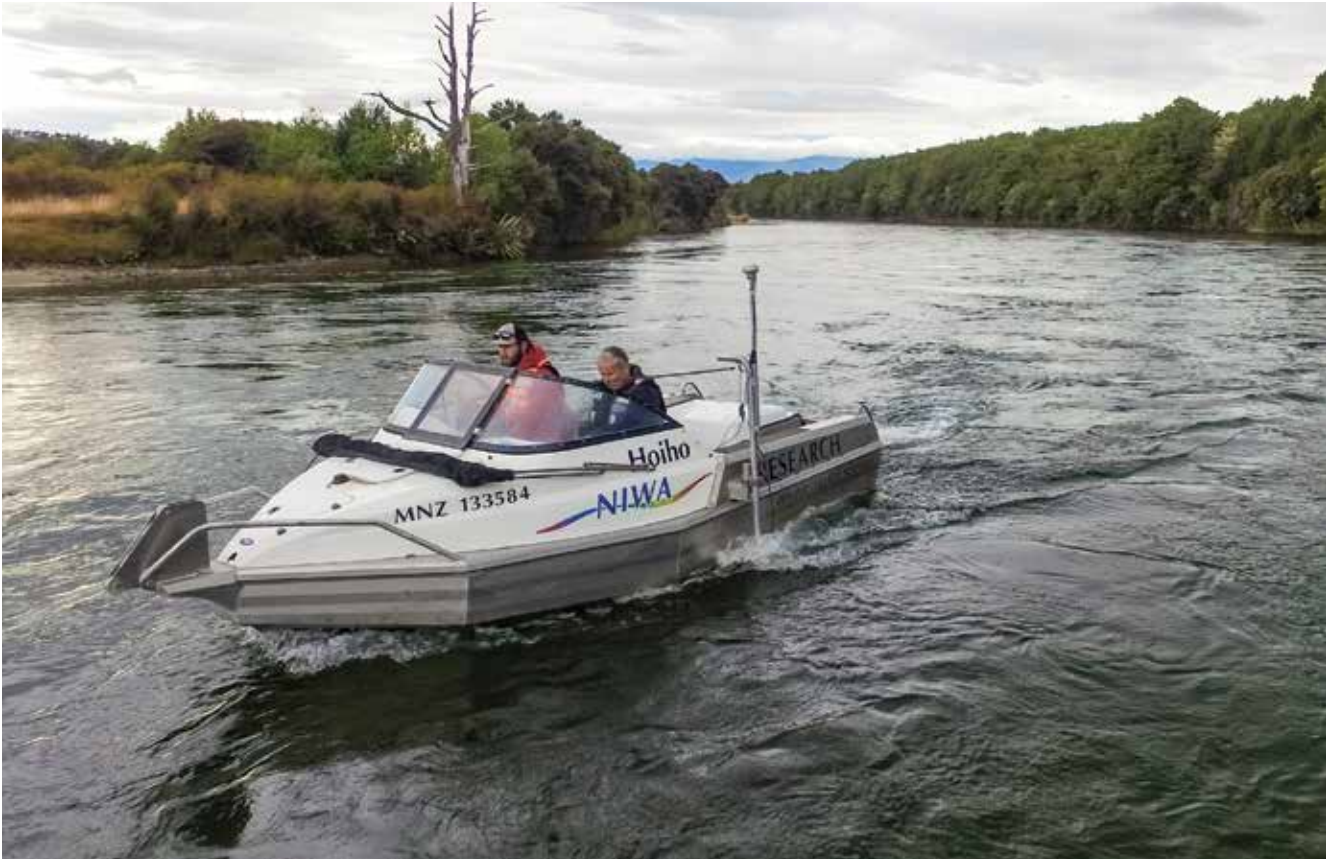
ADCP (Acoustic Doppler Current Profiler) equipment is mounted alongside this small jet boat. To calculate water current velocities the equipment sends out sound waves and measures the reflected signal or echo from particles within the water column and also the river bed for depth. (Dave Allen)
